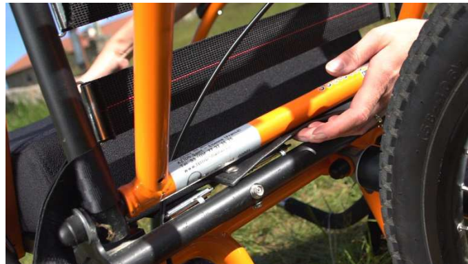
14- Place it under the seat and press the stud
