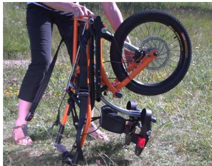
9- Swing the Joëlette tu put it on its supports
