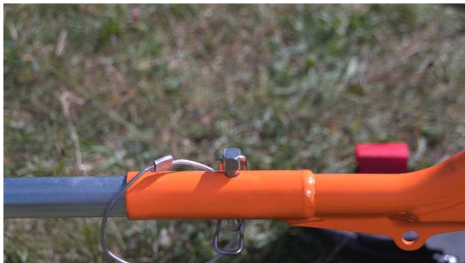
17- Lock the arms with the safety pin
