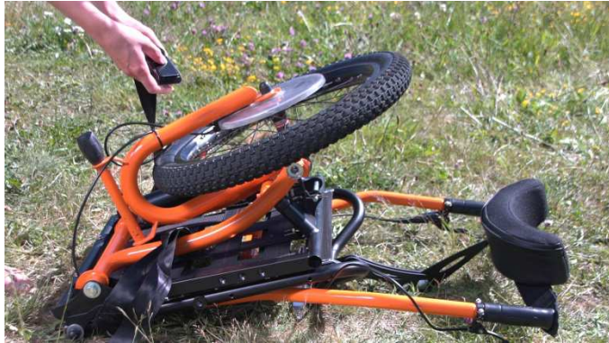
1- Remove the belt and clear the headrest
