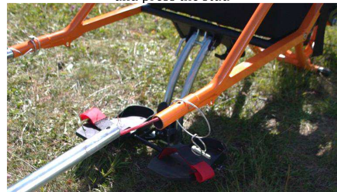
16- Unfold the arms and fit the two parts
