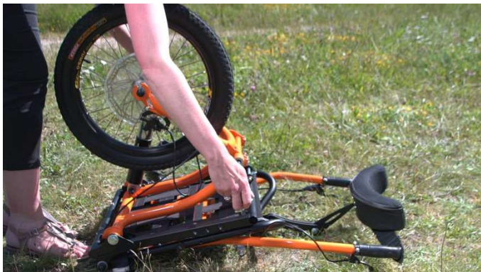
3- Place the pin again in its axle and put the security pin back
