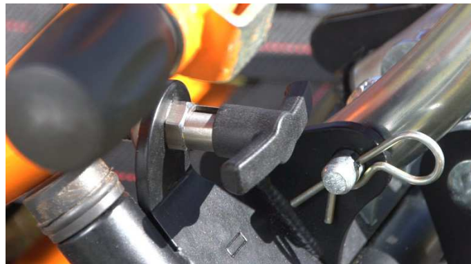
8- Place the indexing finger in a horizontal position
