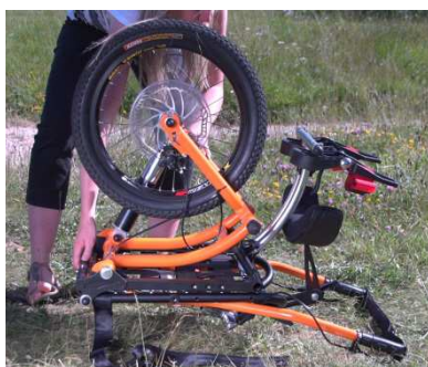
7- Put the axle back in its compartment and lock it. Then, put the security pin back.
