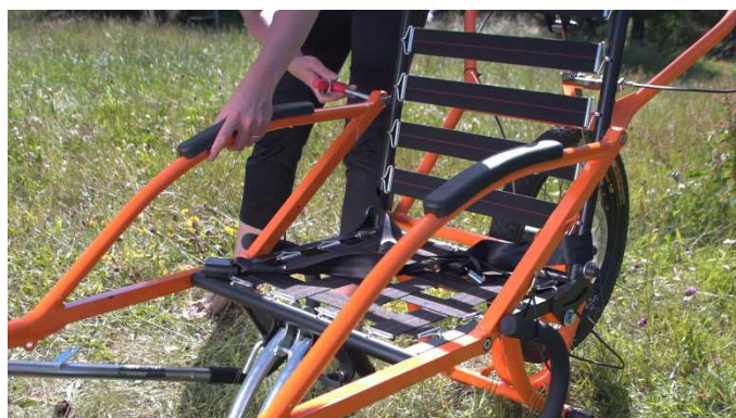
12- Do the same for the seat and tighten the screws. Proceed the same way on the second arm.
